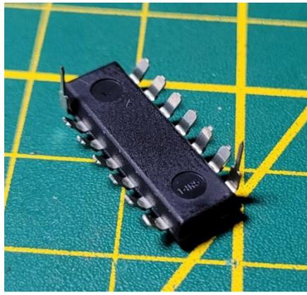
Then solder this chip on top of the U45 chip on the motherboard. Make sure that you correctly position the new chip before soldering. Put some solder onto the pins 1 to 6 - this will be necessary to solder wires to them later.
